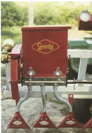
**GANDY** offers a variety of granular applicators. A flow control rotor delivers a constant supply of granules into a delivery tube, through to a ro-bander. The ro-bander spreads the granules in a width of 0.1 - 0.4m. Driving speed further controls rate.
