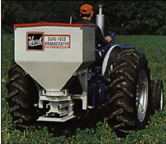
Various models of tractor mounted **HERD** spreaders are available with three-point hitch for easy attachment to tractors. Product hopper capacity ranges from 90 Kg up to 550 Kg depending on the model. For further information go to [www.herdseeder.com](http://www.herdseeder.com).
