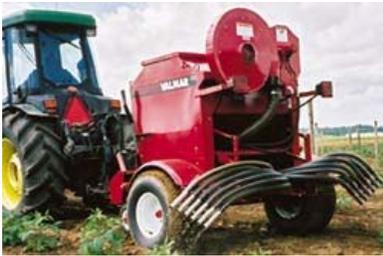
The **VALMAR** Model 1255 Pull type broadcaster has evolved into a multi-use applicator. With the appropriate options, one machine can broadcast inter-row up to 2.2 meters or apply a surface band 30-75 cm row spacing up to 3 meters. Broadcast booms are also available to apply in 4.8 or 6.0 meter swaths.
